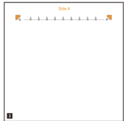
3 Run 10 m of wire rope through the fixings of one side.
