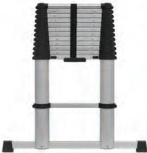
A brilliant quality design. The ladder extends from just 910mm to 3810mm, 13-Tread Aluminium Telescopic Ladder EN 131. Maximum capacity 150kg, Net weight 15.3kg. Additional carriage charges may apply.
