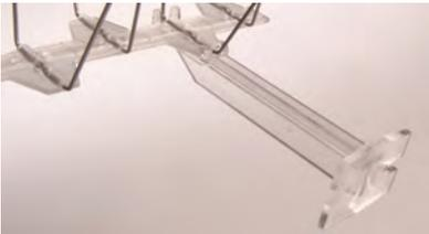
Aviclips for Windows fit securely onto the base of Avipoint™ P20, P32 and G20 Bird Spikes. They allow the spike strips to be easily secured onto window frames using Avifix White adhesive or screws. These clips are extremely useful as they allow the spikes to protect the window sill without hindering the operation of the window. Two clips are required per Avipoint™ strip.
