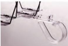
Aviclips for Beams fit securely onto the base of Avipoint™ P14, P20, P32 and G20 bird spikes. They allow the spike strips to be clipped onto beams up to 35 mm thick and 40 mm to 230 mm deep. The clips should be used where you cannot glue the Avipoint™ Bird Spikes onto the Beam. The clips and attached spikes can be removed if access to the beam is required for maintenance, cleaning or painting. Two clips are required per Avipoint™ strip.
