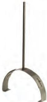
This Bracket holds the straining wire above a roof ridge. Half-Round Ridge Brackets rods on the brackets are 450 mm in height. Half-Round Brackets are designed to clamp under the edge of the ridge tiles.
