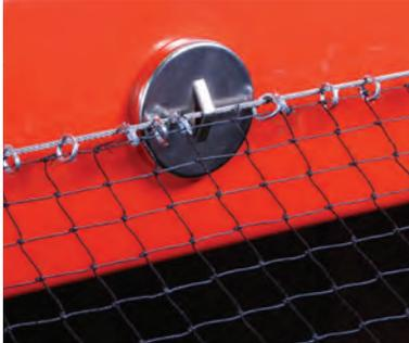
Net Magnets come in handy when drilling or screwing is not an option. These magnets are extremely quick to secure in place and can be useful for following contours of a metal substrate with a wire cable. Use Caution as these are not as strong as screwed fasteners. Holds up to 7 kg.
