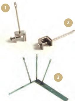
Gutter Posts are for clamping Bird Wire onto vertical flanges and gutters. The Beam Clamps are designed for horizontal flanges, girders and beams. Triangular and Half-Round Ridge Brackets are used to proof roof ridges with Bird Wire. Both can be secured with Blind Anchor Rivets and Avifix.
