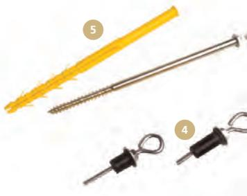
Nylon Cladding Bolts form a secure fastening into thin metal or plastic sheeting. Simply drill a 13 mm hole, push the nylon 'nut' up to its collar into the cladding, then clamp it in place by screwing in the eyebolt - all done from the outside.
