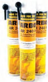
Fire-rated expanding Polyurethane Foam has been tested in horizontal and vertical applications to BS476 Part 20. Suitable for sealing joints where fire integrity and insulation is required e.g. walls, floors and partitioning. Perimeter joints around door and window frames and service penetrations.
