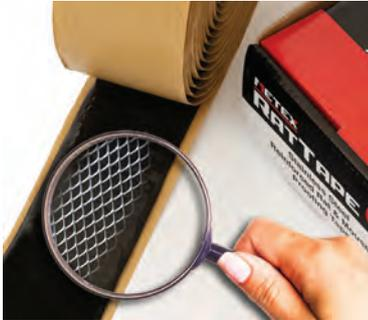
A seriously tough rat and mouse proofing tape, two layers of butyl tape sandwich a dense stainless steel mesh core. It is incredibly flexible, virtually impenetrable and has excellent adhesion to most building materials and may be overpainted to blend with its surroundings.
