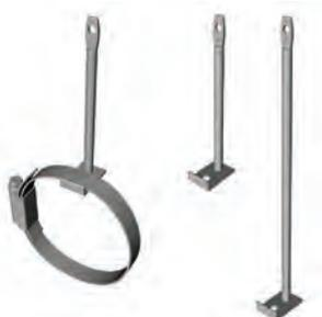
Rail Clamps a popular way of supporting Bird Wire on rails and pipes. These new two-part Rail Clamps and Rail Clamp Posts allow more functionality: You can fasten the clamp tightening screw in any position that best suits the installation; the Rail Clamp Posts can be used separately for installation onto cladding by screwing in place through the 5 mm fixing hole in the base.
