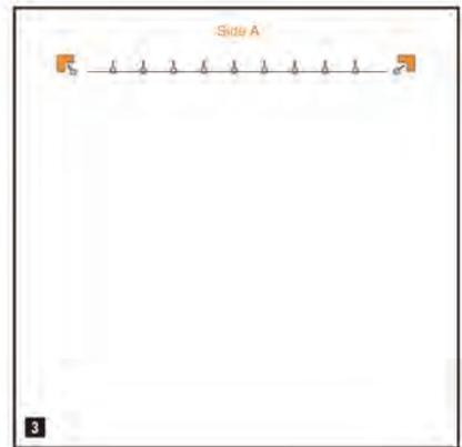
3 Run 10 m of wire rope through the fixings of one side.
