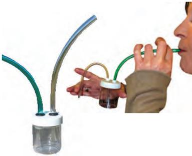
Convenient and easy way to collect samples in the field. Simply suck on the tube whilst placing the other straw over the insect (will stop you receiving a mouthful!) and you can professionally collect insects large and small for identification etc, without damaging them.
