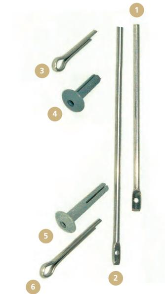
All Bird Posts are made from stainless steel and are installed by knocking them into the nylon Anchor Rivets. Split Pins are used instead of Bird Posts in circumstances where you have a vertical wall at the end of a wire; these are also inserted into the Anchor Rivets.
