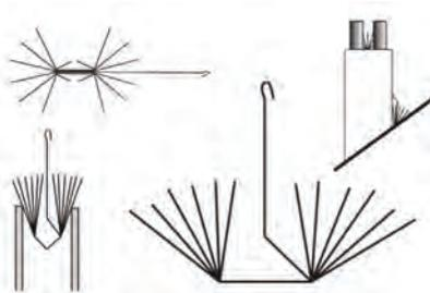
Heavy-duty spike designed to prevent seagulls from nesting in small areas on roofs. Made from 3 mm stainless steel rods, it can be bent in place to protect areas such as chimney pots, between the slope of a roof and the chimney stack. Recommended to be used in conjunction with Avipoint G20 Bird Spikes. Supplied flat packed.
