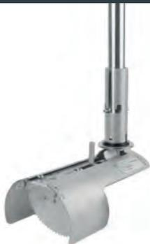
Stainless Steel Nordisk TX11 twin flap Rat Blocker, 100mm (4 inches) diameter and 150mm (6 inches) are industrial grade, suitable for clay, PVC & cast iron pipe systems to suit installation within either an outlet or inlet of a drainage chamber. Other sizes are available.
