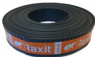
The patented seal is developed in the flexible and durable material Santoprene™. The 3.2 mm thick Santoprene™ is reinforced with embedded acid-resistant steel wires, which makes it impossible for rodents and other pests to penetrate through it. Available in 1 metre replacement strips.
