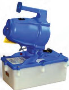
ULV/misting electric portable aerosol applicator, dispenses both OIL and WATER-BASED liquids. Adjustable output up to 19 litres/h. Available with tank float valve for continuous operation. Particle size: 5-50 microns (mmD). Tank capacity: 3.8 L. Weight: 3 Kg. Metering valve to control output and droplet size.
