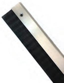
Raxit's patented seal is developed in the flexible and durable material Santoprene™. The 3,2 mm wide Santoprene™ is reinforced with embedded acid-resistant steel wires, which making it impossible for rodents and other pests to penetrate through it. The seal is corrugated to ensure the inlaid steel wires do not slide. The aluminium strip is produced in anodized aluminium (6063).
