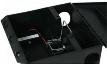
The latest in electronic switch technology: Remote monitoring for both rat and mouse traps. Unit consists of a remote monitoring system that sends a message to your smartphone when a trap is triggered. This alert allows the user to schedule visits to premises once traps have been triggered to remove the rodent and reset the traps. Multiple traps can be set via the control module. Ideal device to increase the daily productivity, customer visits and rodent control success rates.
