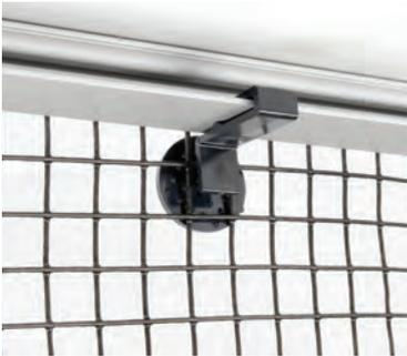
This innovative system is designed specifically to keep all creatures from getting under solar arrays, protecting the roof, wiring and equipment from their damage. This non-penetrating system is fast and easy to install, and can be removed for service. The Solar Mesh Clips are recommended every 18 inches. Tin Snips and other basic tools required for Installation.
