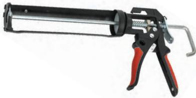
This heavy-duty caulk gun is suitable for 310 ml cartridges with a length of up to 220 mm. The handle has a built in caulk tube cutter so no additional cutting tools are required, just simply insert the tip between the blade and squeeze the handle. A tip piercer/cleaner also features to clear dried product from the end nozzle or tip.
