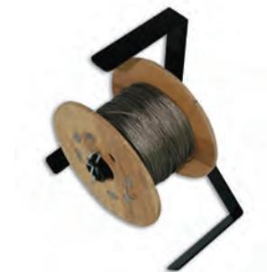
The Wire Reel Holder has been specifically designed to hold wire rope reels for bird work. It allows you to pull off the wire as required to help avoid wire tangling or reels rolling away. The reel simply drops on to the centre spindle, and the retaining pin clips in place to hold it on. This handy tool can save you a lot of installation time and frustration.
